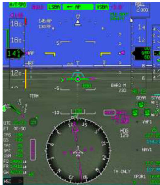
Figure 3: Experimental display – GBAS CAT II/III approach in Atlantic City
