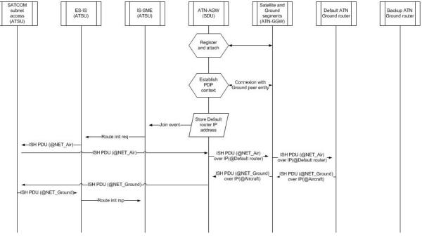
Figure 5: "ATN join" sequence diagram (with default AGR)
