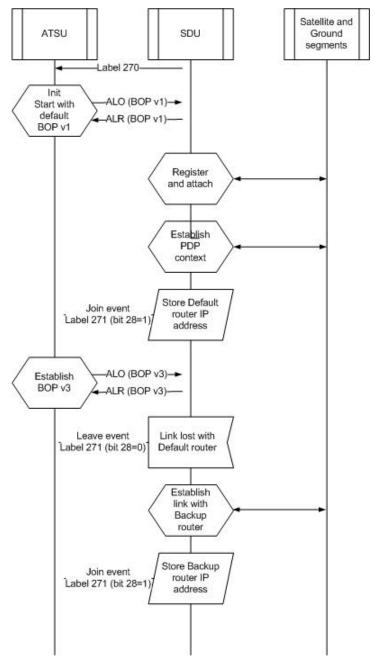
Figure 7: Typical "P15.2.5 Iris Precursor" sequence diagram (Williamsburg protocol)
