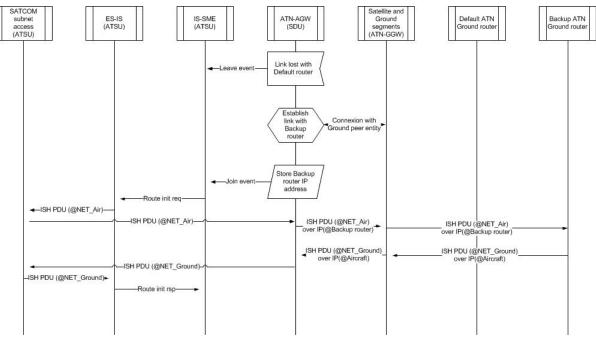
Figure 6: "ATN leave/join" sequence diagram (handover to backup AGR)
