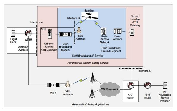
Figure 1: End-End System Architectural Concept
