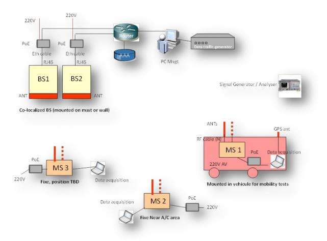
Figure 14: Thales equipment foreseen setup for Airport ground tests
