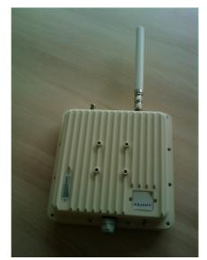
Figure 12: Mobile Station equipped with a collinear antenna
