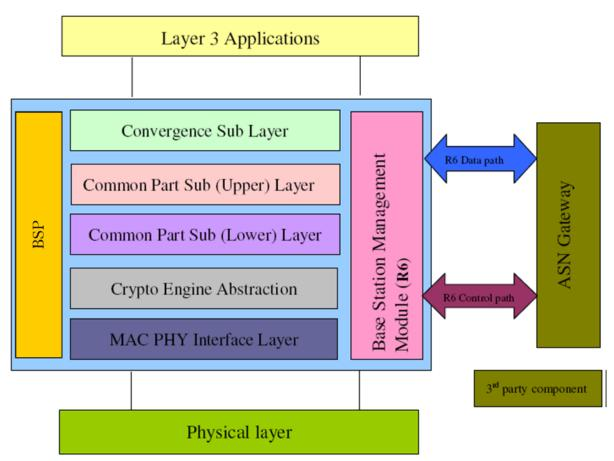
Figure 6: IF3 Internal Switch <--> ASN-GW
