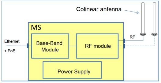
Figure 13: Mobile Station architecture and interfaces
