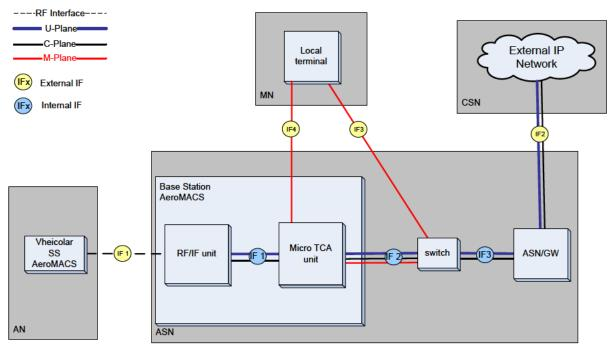
Figure 5: Selex ES ASN Internal and External Interfaces
