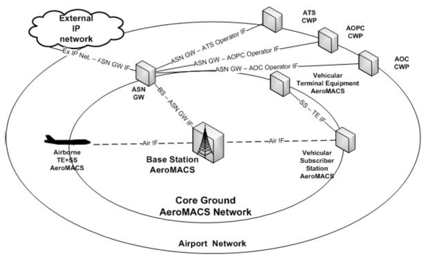
Figure 1: AeroMACS Network Reference Model
