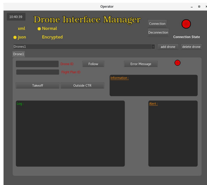
Figure 18: Mock-up of collaborative interface for drone pilots
